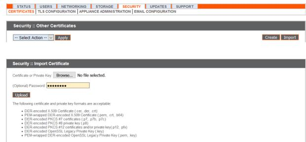
Your signed certificate should now appear in the **Security :: Other Certificates** section. If the new certificate shows a warning beneath its name, this typically means the intermediate and/or root certificates from the CA have not been imported. The components of the certificate chain can be identified as follows:
